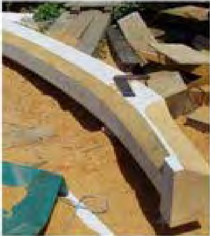
Top L. First outer wale plank entry runs.
